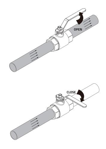
Figure 3.1 Rotation Direction for CLOSED and OPEN position
