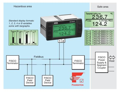
The BA488CF-F Fieldbus Display is an intrinsically safe instrument that can display up to eight fieldbus process variables. Eleven selectable standard screen formats contain one, two, three, four or eight variables, with units of measurement, tag descriptions and bargraphs on some screens.
