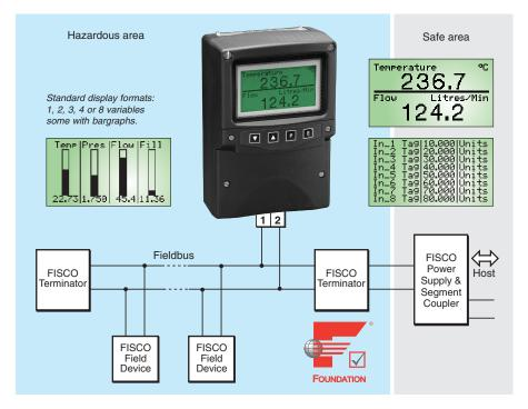
The BA484DF-F Fieldbus Display is an intrinsically safe instrument that can display up to eight fieldbus process variables. Eleven selectable standard screen formats contain one, two, three, four or eight variables, with units of measurement, tag descriptions and bargraphs on some screens.
